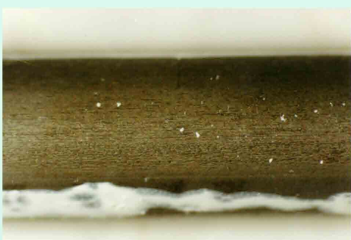
Surface after mechanical descaling without guidance marks
