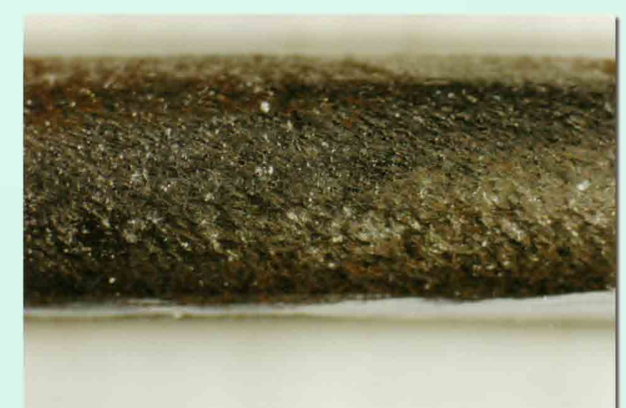
Strongly deformed surface after brushing
